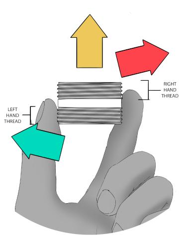
The diagram to the left shows how to recognise the two thread directions of a double threaded nipple used to join cast iron radiators.
